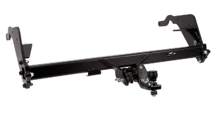
TOW BAR 1,200kg braked, 660kg unbraked towing capacity, with a 50kg tow ball download limit.
